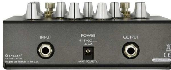
**INPUT** – Pedal input, nominally instrument level but can accept line level as well. When operating at line level, greater headroom is available with a 12V, 15V or 18V power supply. Input impedance is 1M ohm.
